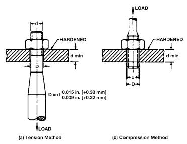
FIG. 1 Proof Load Testing-Nuts
