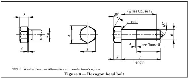
8.1.2 The standard thread lengths shall be based on the formulae set out in Table 4 in accordance with BS 7375.
