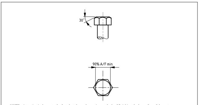
NOTE Attention is drawn to the fact that these alternative methods of finishing the lower face of the nut are associated both with the nominal size and the particular method of manufacture. A request by the purchaser for a specific type of finish limits the manufacturing processes available, and it is therefore recommended that the purchaser avoids making such a request unless circumstances fully justify it.
