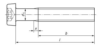
NOTE The shank diameter,  $d_{\rm S}$ , is approximately equal to the pitch diameter or equal to the major thread diameter.
