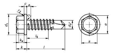
a The function of the drilling point (diameter  $d_{\rm p}$ ) is specified in ISO 10666.
